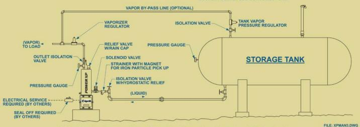
Note: No check valves in liquid line; liquid must be able to flow in both directions.
